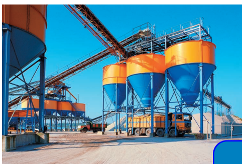
Photo 5.2 The storage tanks shown are bodies of revolution. Thus, their surface areas and volumes can be determined using the theorems of Pappus-Guldinus.
