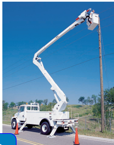
10.1 The forces exerted by the hydraulic cylinders to position the bucket lift shown can be effectively determined using the method of virtual work since a simple relation exists among the displacements of the points of application of the forces acting on the members of the lift.
