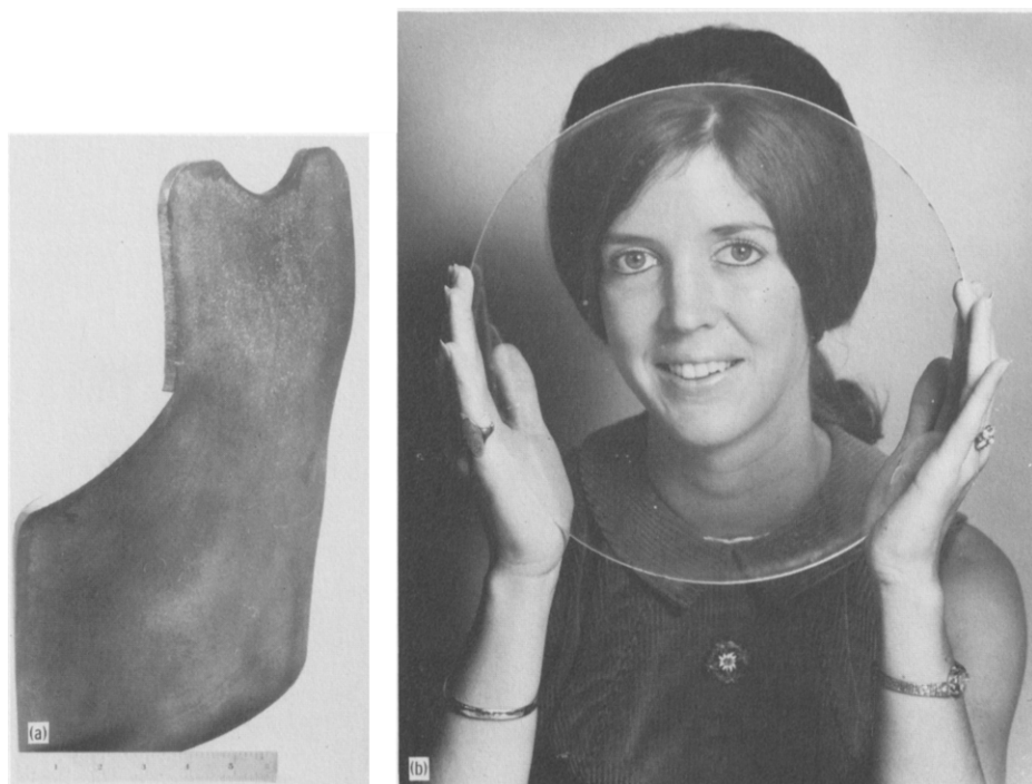
Fig. 1. (a) Hot pressed B 4 C body armor plate. Courtesy Norton Co., Worcester, Massachusetts. (b) Hot pressed transparent polycrystalline MgO 0.25 inches thick. Courtesy AVCO Systems Division, Wilmington, Massachusetts.
