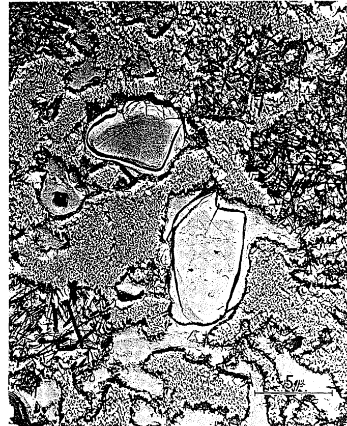
Fig. 11.14. Electron micrograph of electrical insulator porcelain (etched 10 sec, 0°C, 40% HF, silica replica. Courtesy S. T. Lundin.
