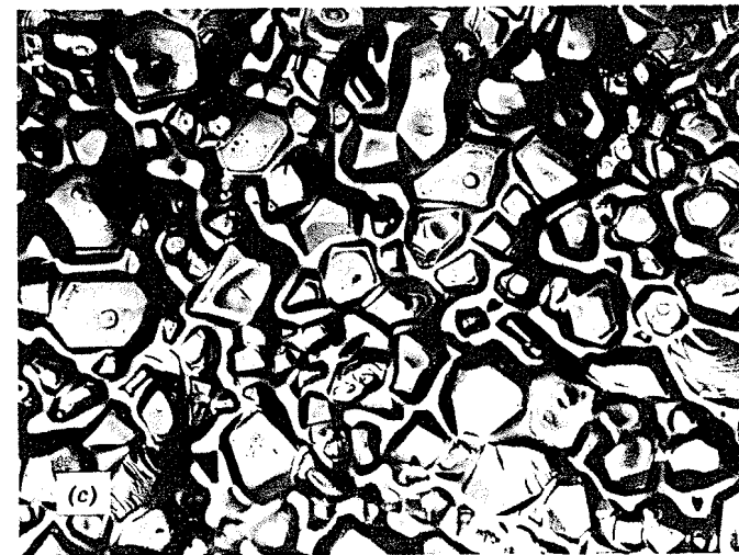
Fig. 10.40. (a) Surface of solid-liquid composite with varying amounts of liquid phase. (b) Drop of liquid between two solid spheres exerts pressure to pull them together. (c) Surface of forsterite ceramic showing liquid capillary depression between crystals.
