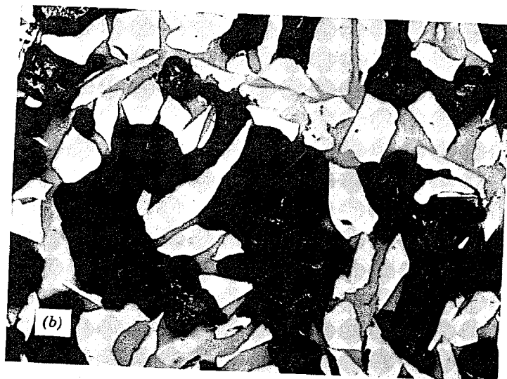
Fig. 11.33. Abrasive products. (a) Section of silicon carbide wheel, unetched (50 \times ); (b) aluminum oxide wheel, unetched (100 \times ). In both light area is grain, gray area bond, and dark area porosity. Courtesy A. Sidhwa.
