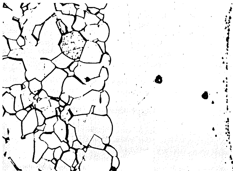
Fig. 10.11. Growth of a large \text{Al}_2\text{O}_3 crystal into a matrix of uniformly sized grains (495 \times ). Compare with Fig. 10.4. Courtesy R. L. Coble.
