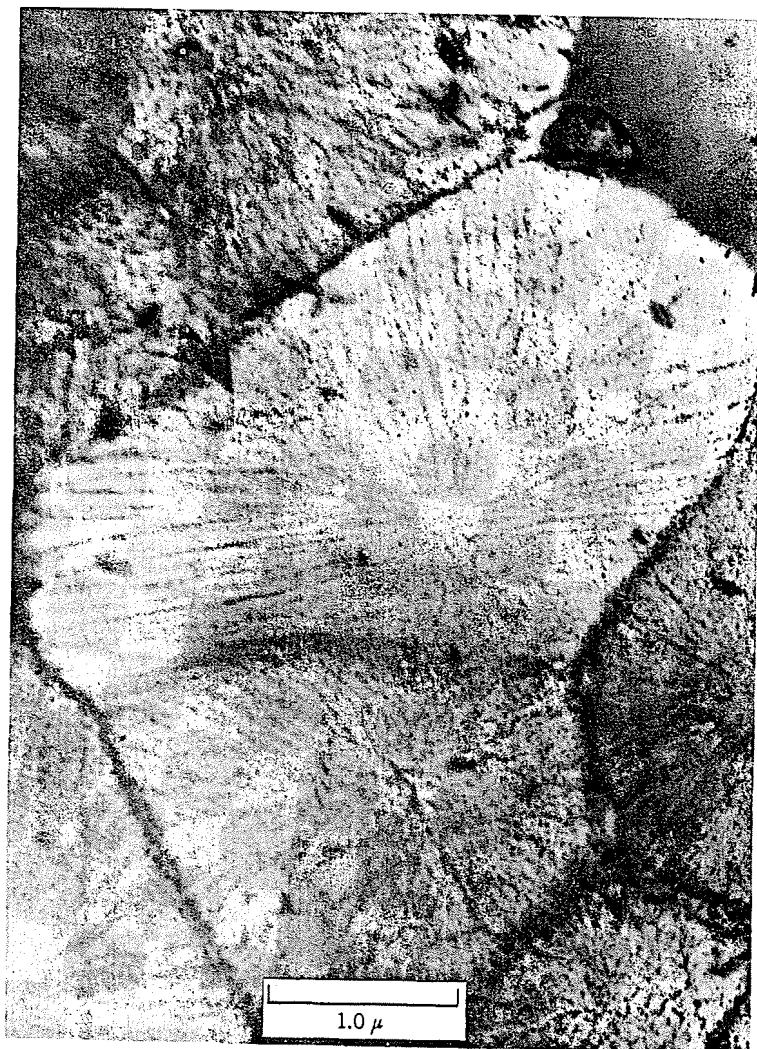
Fig. 8.29. Submicrostructure in \text{Li}_2\text{O}-\text{Al}_2\text{O}_3-\text{SiO}_2 glass-ceramic heated rapidly to 875^\circ\text{C} and held for 25 min. From P. E. Doherty in R. M. Fulrath and J. A. Pask, Eds., Ceramic Microstructures , John Wiley & Sons, Inc., New York, 1968, pp. 161-185.
