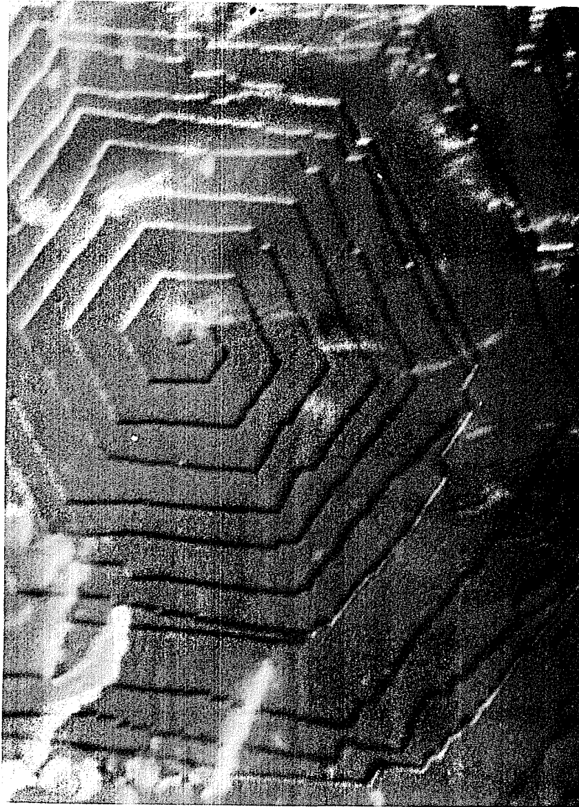
Fig. 8.10. Growth spiral on cadmium iodide crystals growing from water solution. Interference contrast micrograph at 1025 \times . Courtesy Dr. K. A. Jackson, Bell Telephone Laboratories.
