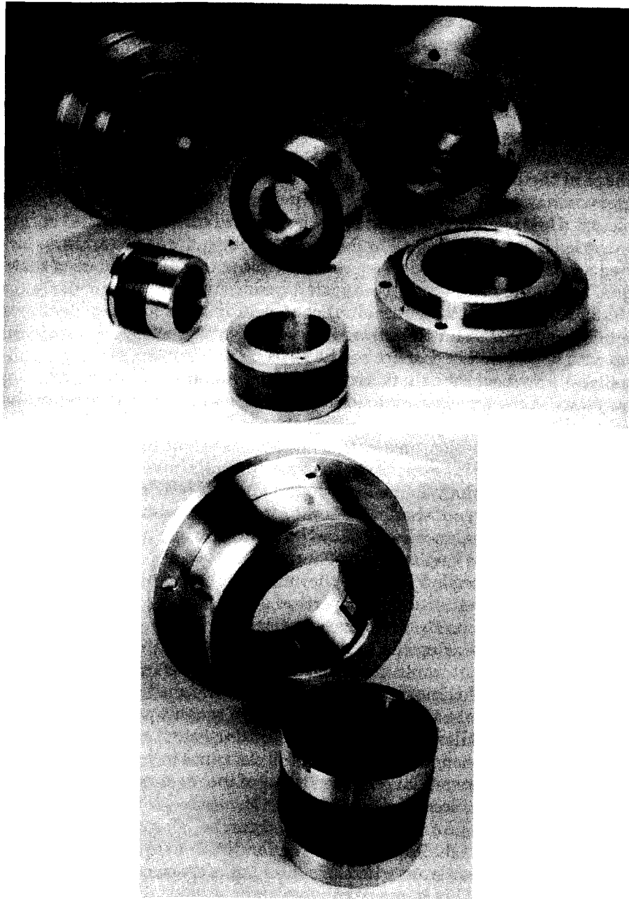
Figure 4-8. Application of ceramics to journal bearings: above , typical pump set of ceramic bearings; below , ceramic tilting pad radial bearing and associated shaft sleeves. Courtesy Federal-Mogul Bearings Group.
