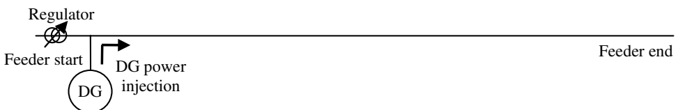
Fig. 19.10. Circuit configuration with the DG at downstream of a regulator used to analyze the voltage along the feeder.
