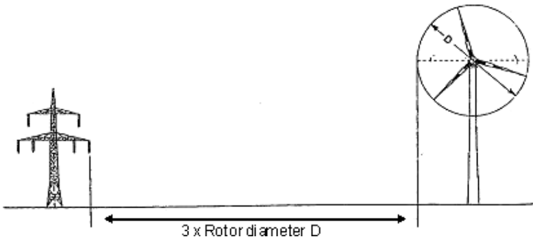
Fig. 7.17. Example of 3D for undamped lines. 21
