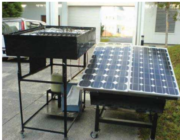
Figure 10.15 Hybrid solar thermoelectric-adsorption cooling system. (From Abdullah et al. 2009 [32].)
