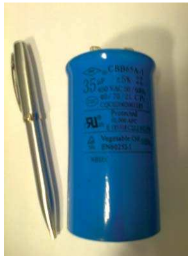
Figure 5.17 A typical capacitor. This capacitor is designed with a capacity of 35\mu\text{F} at 450 VAC, suitable for air-conditioning unit application. (Courtesy of author.)
