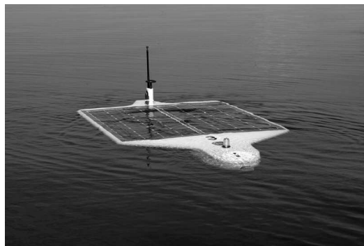
FIGURE 1.104 (See color insert following page 80.) SAUV II. (Courtesy of Solar Powered Autonomous Underwater Vehicle (SAUV II), Falmouth Scientific, Inc., available online: http://www.falmouth.com/DataSheets/SAUV.pdf )
