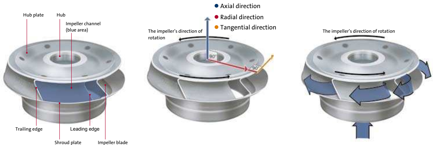
Figure 1.5: The impeller components, definitions of directions and flow relative to the impeller.
