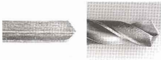
FIGURE 14-10 Straight-flute drill (left) and "dubbed" drill (right) used for drilling plastics.
