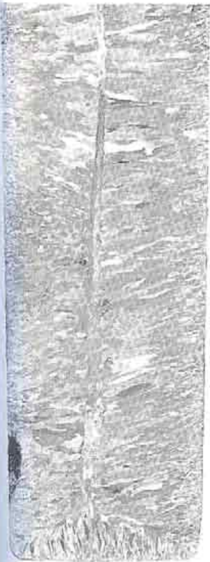
FIGURE 11-5 Internal structure of a cast metal bar showing the chill zone at the periphery, columnar grains growing toward the center, and a central shrinkage cavity.
