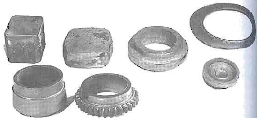
FIGURE 18-14 Comparison of conventional forging and the forging of a powder metallurgy preform to produce a gear blank (or gear). Moving left to right, the top sequence shows the sheared stock, upset section, forged blank, and exterior and interior scrap associated with conventional forging. The finished gear is generally machined from the blank with additional generation of scrap. The bottom pieces are the powder metallurgy preform and forged gear produced entirely without scrap by P/M forging (Courtesy of GKN Sinter Metals, Auburn Hills, MI)
