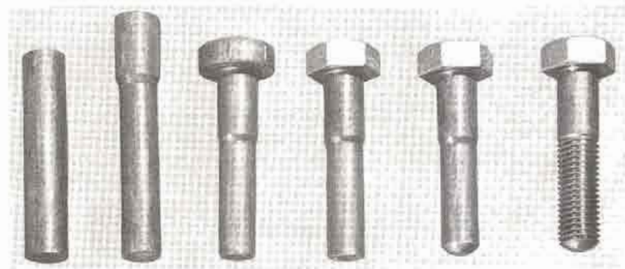
FIGURE 16-45 Steps in the forming of a bolt by cold extrusion, cold heading, and thread rolling. (Courtesy of National Machinery Co., Tiffin, OH.)
