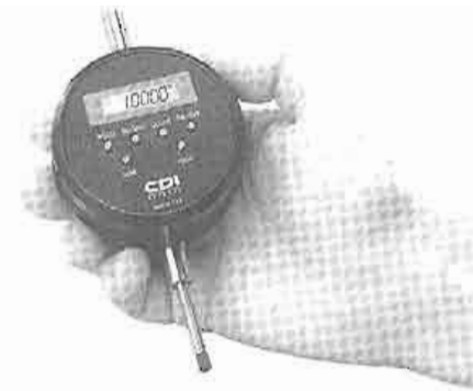
FIGURE 10-41 Digital dial indicator with 1-in. range and 0.0001-in. accuracy. (Courtesy of CDI.)
