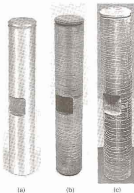
FIGURE 10-45 Front-axle king pin for a truck. (a) As manufactured and apparently sound; (b) inspected under conventional magnetic particle inspection to reveal numerous grinding-induced cracks; (c) fluorescent particles and ultraviolet light make the cracks even more visible. (Courtesy of Magnaflux Corporation.)
