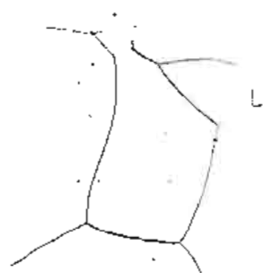
FIGURE 3-11 Photomicrograph of alpha ferrite (essentially pure iron) showing grains and grain boundaries; (Courtesy of United States Steel Corp., Pittsburgh, PA)
