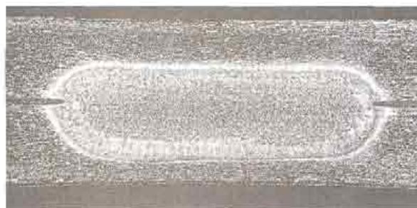
FIGURE 32-5 A spot-weld nugget between two sheets of 1.3-mm (0.05-in.) aluminum alloy. The nugget is not symmetrical because the radius of the upper electrode is greater than that of the lower electrode. (Courtesy Lockheed Martin Corporation, Bethesda, MD.)
