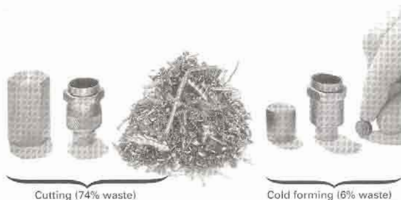
FIGURE 16-48 Manufacture of a spark plug body: (left) by machining from hexagonal bar stock; (right) by cold forming. Note the reduction in waste. (Courtesy of National Machinery Co., Tiffin, OH.)
