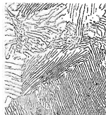
FIGURE 4-12 Pearlite; 1000X. (Courtesy of United States Steel Corp., Pittsburgh, PA.)
