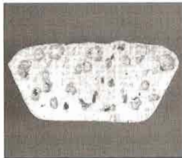
FIGURE 11-8 Demonstration casting made from aluminum that has been saturated in dissolved hydrogen. Note the extensive gas porosity.
