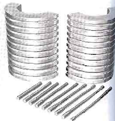
FIGURE 16-19 (Right) Rolls from a roll-forging machine and the various stages in roll forging a part. (Courtesy of Ajax Manufacturing Company, Euclid, OH.)
