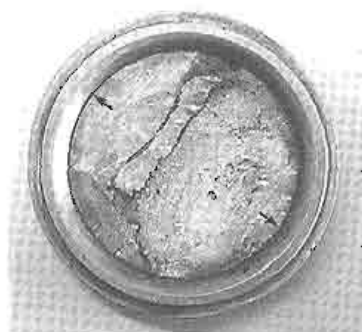
FIGURE 2-28 Progressive fracture of an axle within a ball-bearing ring, starting at two points (arrows).
