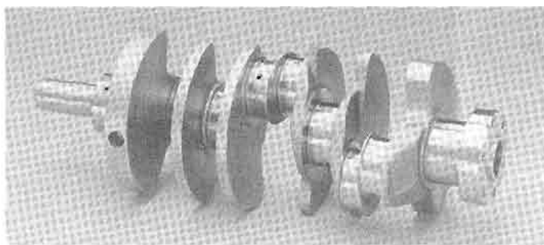
FIGURE 16-15 A forged-and-machined automobile engine crankshaft that has been formed from microalloyed steel. Performance is superior to cranks of cast ductile iron.
