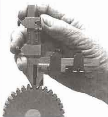
FIGURE 29-27 Using gear-tooth vernier calipers to check the tooth thickness at the pitch circle.
