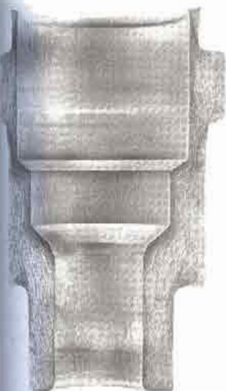
FIGURE 16-49 Section of the cold-formed spark plug body of Figure 16-48, etched to reveal the flow lines. The cold-formed structure produces an 18% increase in strength over the machined product. (Courtesy of National Machinery Co., Tiffin, OH.)
