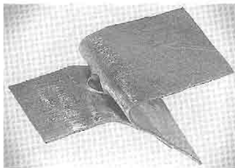
FIGURE 32-6 Tear test of a satisfactory spot weld, showing how failure occurs outside of the weld.
