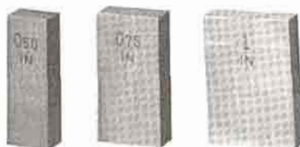
FIGURE 10-3 Standard set of rectangular gage blocks with 0.000050-in. accuracy; three individual blocks are shown.
