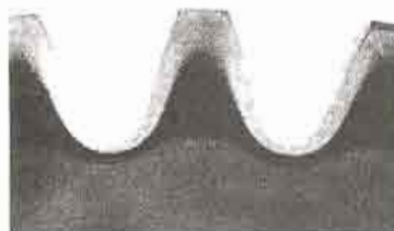
FIGURE 5-23 Section of gear teeth showing induction-hardened surfaces. (Courtesy of Ajax Tocco Magnathermic Corp., Warren, OH.)
