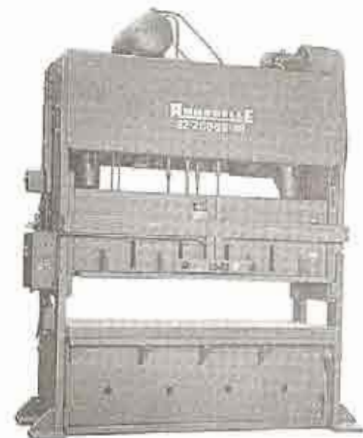
FIGURE 17-61 A 200-ton (1800-kN) straight-sided press. (Courtesy of Rousselle Corporation, West Chicago, IL.)
