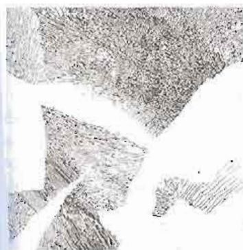
FIGURE 4-13 Photomicrograph of a hypoeutectoid steel showing regions of primary ferrite (white) and pearlite; 500X. (Courtesy of United States Steel Corp., Pittsburgh, PA.)
