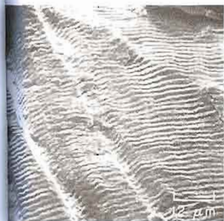
FIGURE 2-29 Fatigue fracture of AISI type 304 stainless steel viewed in a scanning electron microscope at 810X. Well-defined striations are visible. (From "Interpretation of SEM Fractographs," Metals Handbook , Vol. 9, 8th ed., ASM International, Materials Park, OH, 1970, p. 70.)
