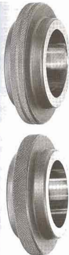
FIGURE 10-36 Go and no-go (on right) ring gages for checking a shaft. (Courtesy of Automation and Measurement Division, Bendix Corporation.)
