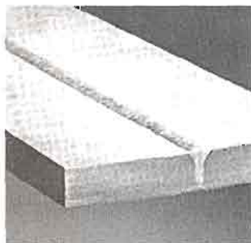
FIGURE 33-4 Laser butt weld of 3-mm (0.125-in.) stainless steel, made at 1.5 m/min with a 1250-watt laser (Courtesy of Coherent, Inc., Santa Clara, CA)
