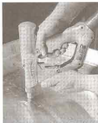
FIGURE 31-22 Making a spot weld by the inert-gas-shielded tungsten arc process. (Courtesy of Air Reduction Company Inc., New York, NY)
