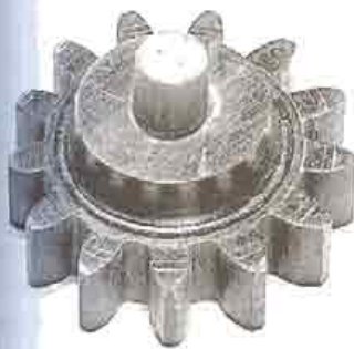
FIGURE 12-2 Single-piece pattern for a pinion gear.
