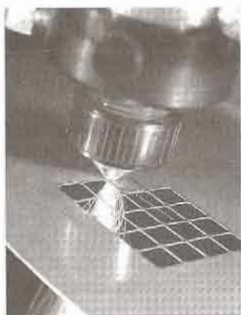
FIGURE 31-27 Cutting sheet metal with a plasma torch. (Courtesy of GTE Sylvania, Danvers, MA)
