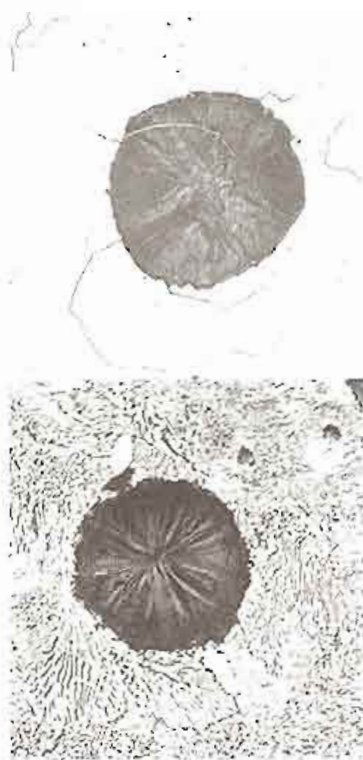
FIGURE 4-18 Ductile cast iron with (a) ferrite matrix and (b) pearlite matrix; 500X. Note the spheroidal shape of the graphite nodule in each photo.
