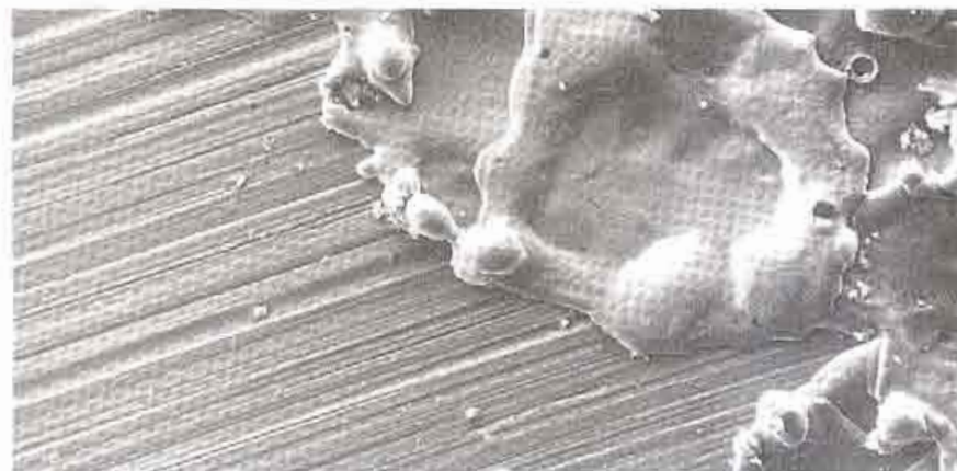
FIGURE 19-24 SEM micrograph of EDM surface (right) on top of a ground surface in steel. The spheroidal nature of debris on the surface is in evidence around the craters (300 \times ).
