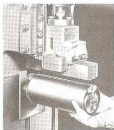
FIGURE 17-60 Making a seam on a horn press. Note the protruding "horn" that replaces the lower press bed. (Courtesy of Niagara Machine & Tool Works, Buffalo, NY.)
