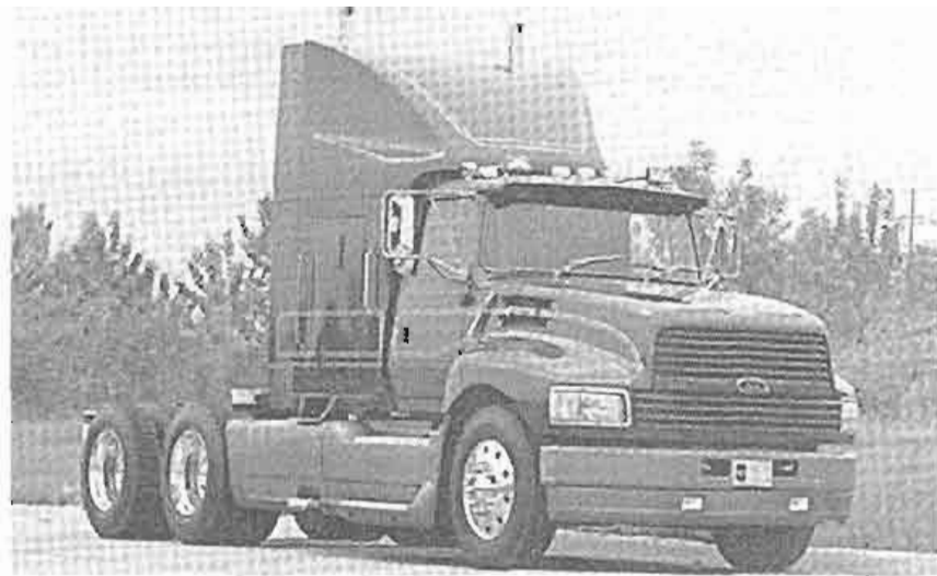
FIGURE 14-24 Aerodynamic styling and smooth surfaces characterize the hood and fender of Ford Motor Company's AeroMax truck. This one-piece panel was produced as a resin-transfer molding by Rockwell International. (Courtesy of ASM International, Metals Park, OH.)
