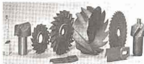
FIGURE 12-27 Group of intricate cutters produced by ceramic mold casting. (Courtesy of Avnet Shaw Division of Avnet, Inc., Phoenix, AZ)
