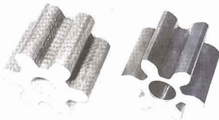
FIGURE 13-13 Gear produced by continuous casting. (Left) As-cast material; (right) after machining. (Courtesy of ASARCO, Tucson, AZ.)
