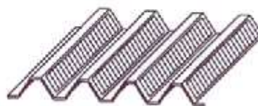
Multi Louvered used in the Microchannel
