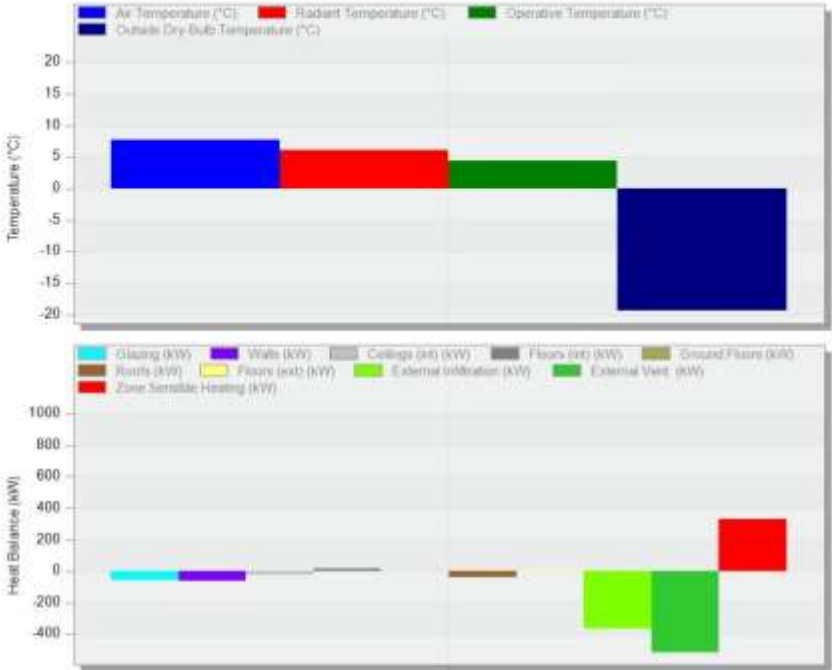
Temperature and Heat Loss Using the thermal break window
