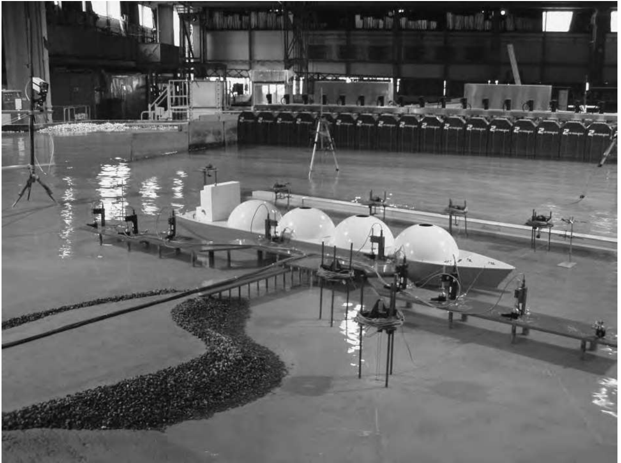
FIGURE 9.3(a) A scaled 135 000 m 3 LNG carrier moored at an undisclosed location in the shelter of a breakwater under multidirectional random wave attack (Image reproduced courtesy of HR Wallingford Group Ltd)
