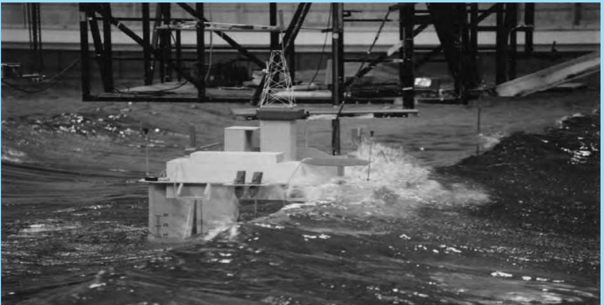
A floating semi-submersible drilling rig being tested in 'design storm' conditions in the Marintek wavebasin, image courtesy of Marintek
