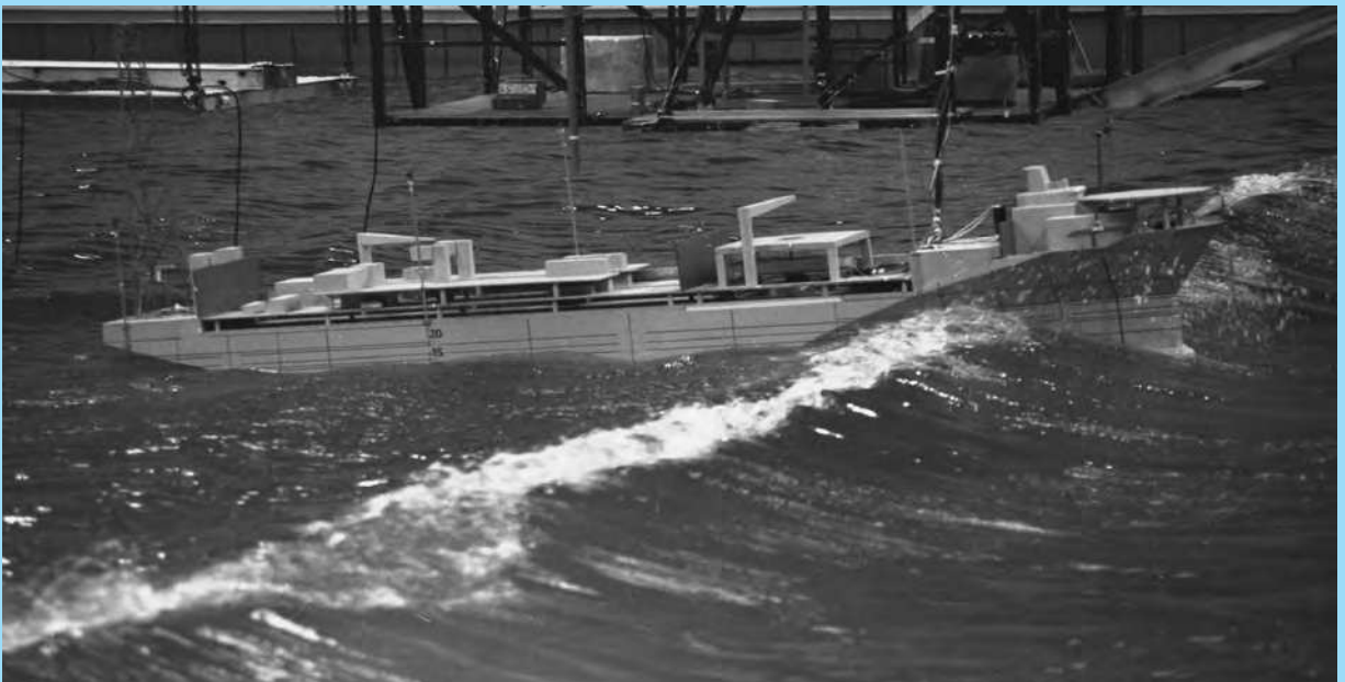
A floating production storage and off-loading (FPSO) vessel model being tested in 'design storm' conditions in the Marintek wave basin, Trondheim, Norway, image courtesy of Marintek.
