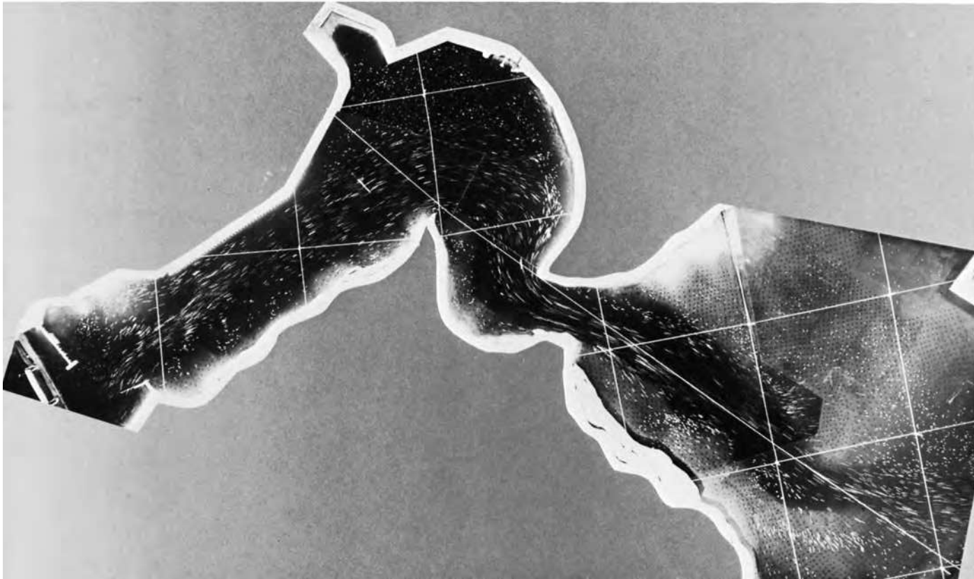
FIGURE 9.3(c) A bird's eye view of a scale model of the entrance channel to Dar-es-Salaam harbour, showing flow patterns at ebb tide. The effect is obtained by scattering confetti on the water and then photographing it with a time exposure. Where the water is moving fastest, the confetti shows as a streak – the longer the streak, the faster the current. By studying results from a series of photographs representing various states of the tide, one is able to calibrate the model so that water flows in the model correspond closely to those recorded on site (Courtesy of UN Development Program, East African Harbours Corp., International Bank for Reconstruction and Development, Bertlin and Partners, Redhill, and The Model Laboratory, Wimpey Laboratory, Middlesex)
