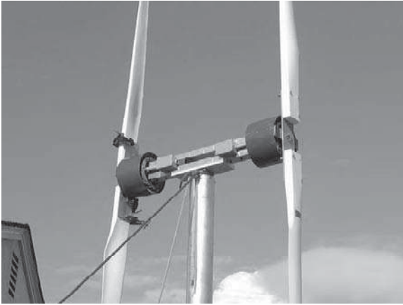
FIGURE 19.13 Assembled contrarotating wind turbine system.
