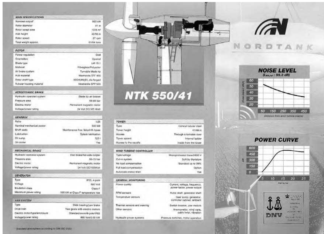
FIGURE 4.8 Technical data sheet of a 550-kW/41-m diameter wind turbine, with power level and noise level. (From Nordtank Energy Group, Denmark. With permission.)
