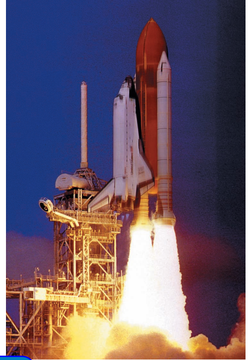
14.3 As the shuttle's booster rockets are fired, the gas particles they eject provide the thrust required for liftoff.
