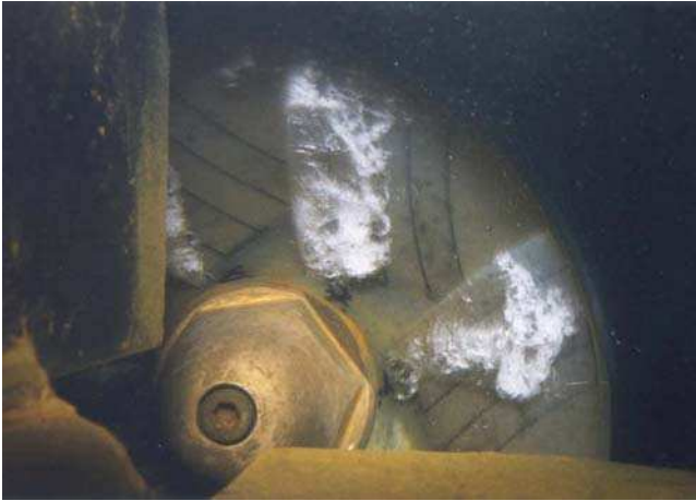
Figure 1.5 Cavitation at the impeller inlet
