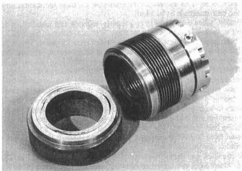
Figure 17-56. Wear of hard seal faces at high temperature.
