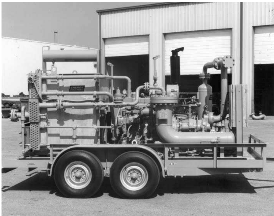
FIGURE 23.10 Trailer-mounted CAT G3304NA/C12 sullair unit.
