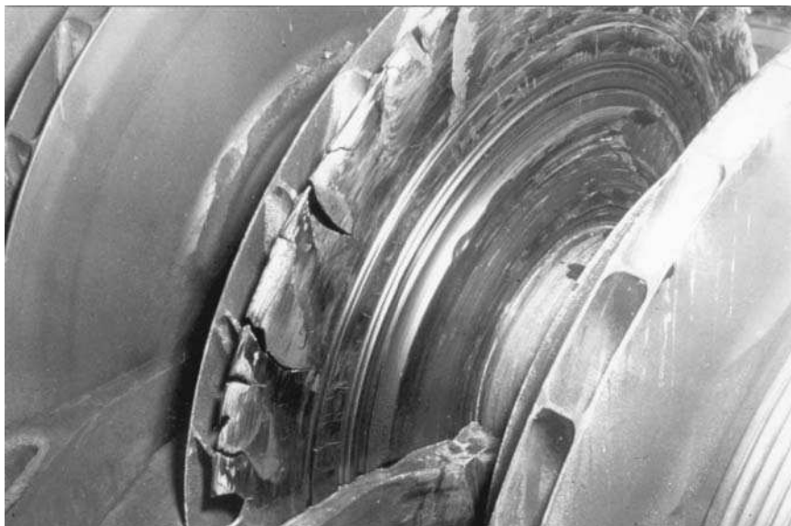
FIGURE 4.53 Damage from surging.
