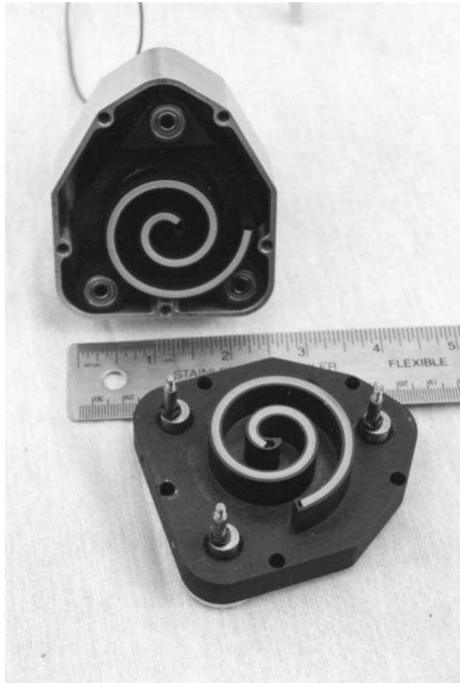
FIGURE 12.4 Typical scroll showing idler shafts.
