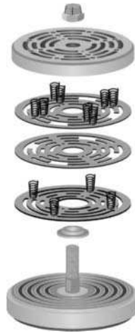
FIGURE 20.5 Double damped valve.
