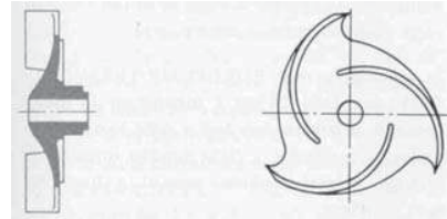
figure 24b axial closed impeller
