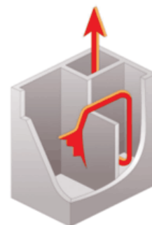
fig ... Flue gas flow
