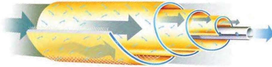
fig ... Water is pumped from the outside through the membrane to come out clean through the central core
