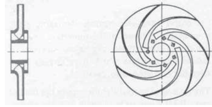
figure 24b axial closed impeller
