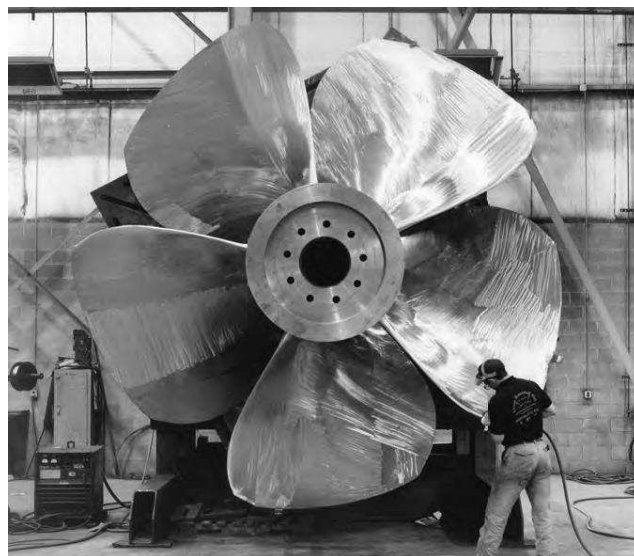
Figure 3. 4 The five-bladed propeller of a Kaplan turbine used at the Warwick hydroelectric power station in Cordele
