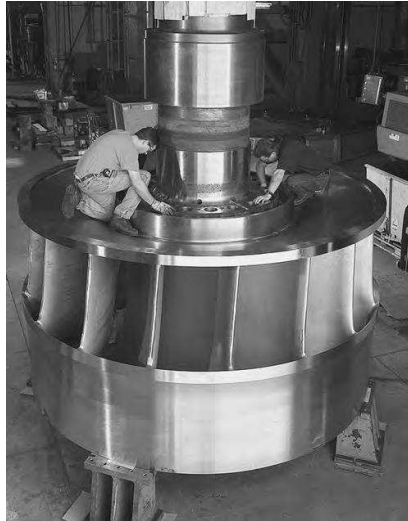
Figure 3. 2 The runner of a Francis radial-flow turbine used at the Round Butte hydroelectric power station in Madras
