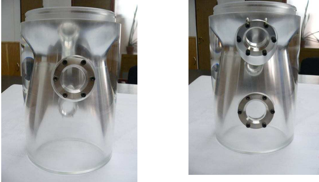
Fig. 9: Actual convergent-divergent test section manufactured from plexiglass.
