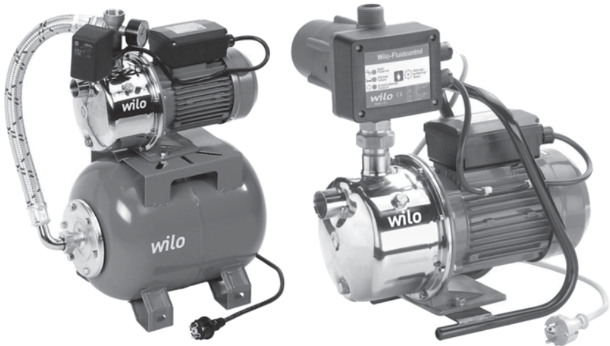
Fig. 7.12 Left domestic pump group with large reservoir and fixed speed; right small reservoir and variable speed (Courtesy Wilo)
