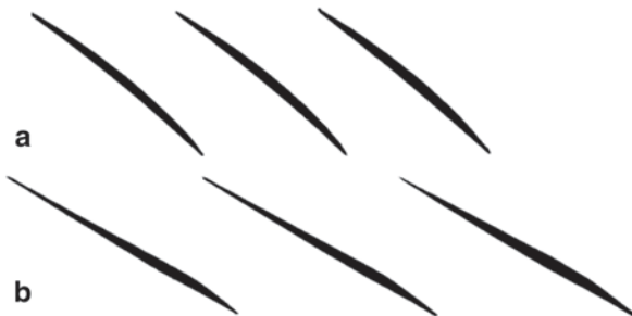
Fig. 13.21 Transonic compressor cascades with a single normal blade passage shock. a Low transonic ( M_1 \sim 1.1 ), convex leading suction side. b Medium transonic ( M_1 \sim 1.2 ), slightly concave leading suction side
