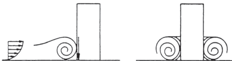
Fig. 13.13 Horseshoe vortex generation; left side view; right back view
