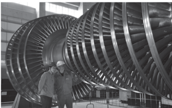
Fig. 6.26 Rotor of the combined HP-IP part of a large impulse type steam turbine. (Courtesy Alstom)
