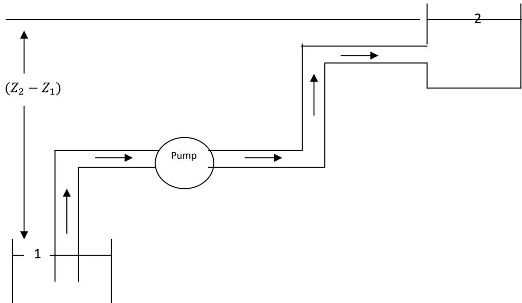
The head ( $H_p$ ) supplied by the pump is given by
