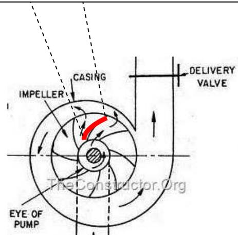
To understand the connectivity between the velocities, for example, consider the velocities of water at the outlet of the pump. At the outlet, we have the following:
