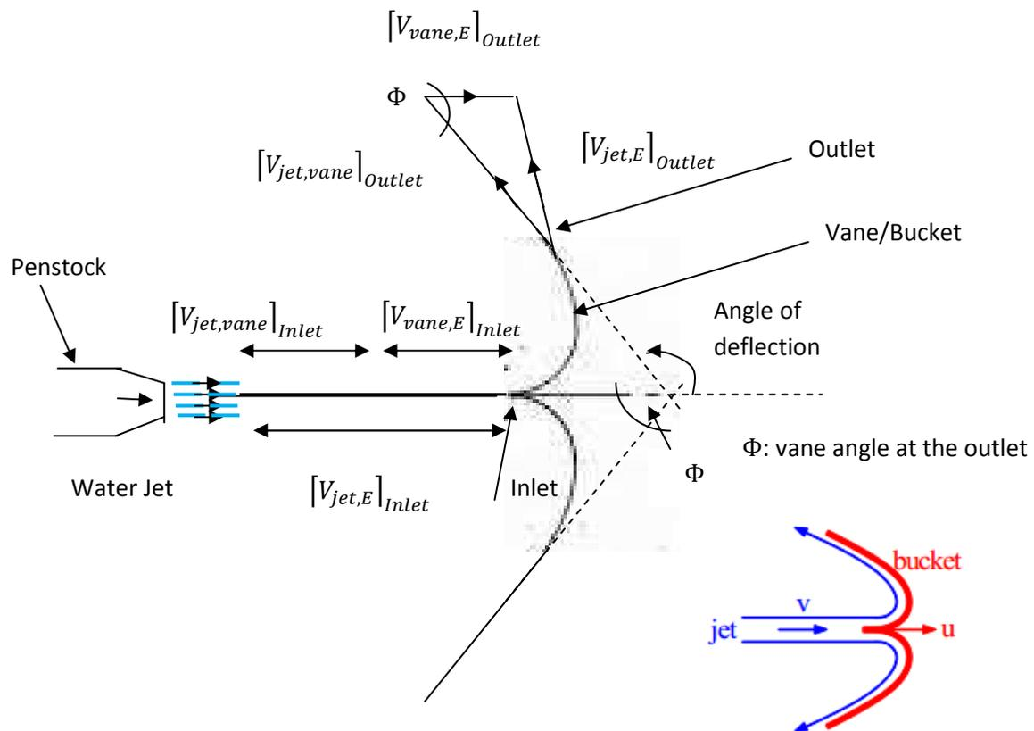
To understand the connectivity between the velocities, for example, consider the velocities of water at the outlet of the turbine. At the outlet, we have the following:
