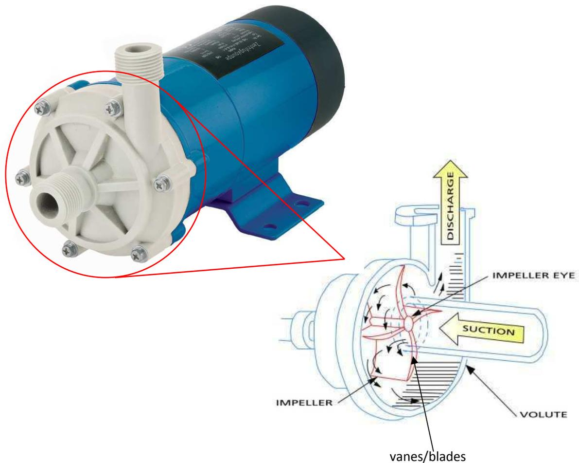
In the operation of a centrifugal pump, the impeller is rotated by an electric motor. The rotation of impeller causes the vanes to impel out the liquid. The liquid that is impelled out by the vanes comes to the out at the outlet.
