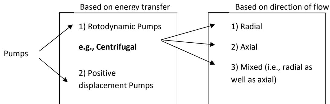
In the operation of a pump, the mechanical action performs two functions. At first, a vacuum is created at the inlet of the pump. This vacuum causes the liquid to flow from the source (e.g., reservoir) into the inlet to the pump. Then, the drawn liquid is delivered to the pump outlet. Due to high capital cost, maintenance cost, grater discharging capacity, etc., centrifugal pumps have become the first choice for industrial uses.
