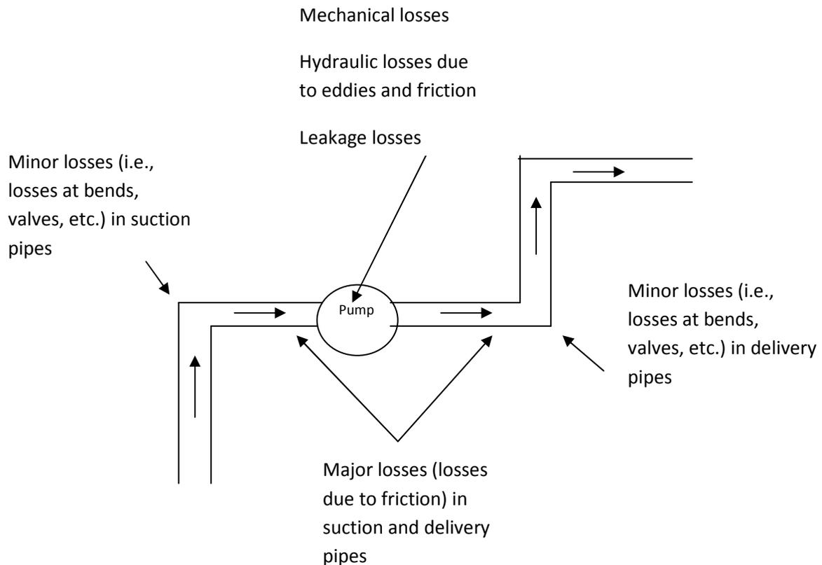
The **losses in the pump** are generally due to eddies, leakages, and bearing friction. The losses due to eddies and friction may arise at the impeller as well as at the vanes of a centrifugal pump. The **losses due to leakage** of liquid, also known as leakage losses, are due to leakage of liquid that happens through the clearances between impeller and casing of a centrifugal pump. The **mechanical losses** are due to bearing friction.
