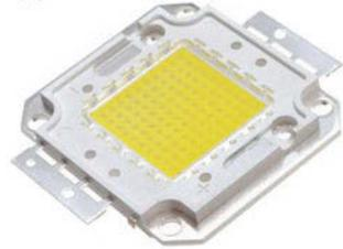
**Fig. 1.14** (a) Blue LED (standard housing). 50 W, 4000 lm (b) warm white and (c) cold white LED ( $45 \times 45$  mm<sup>2</sup>)
