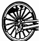
A COUNTERBALANCE OF LOCOMOTIVE DRIVING WHEEL.
