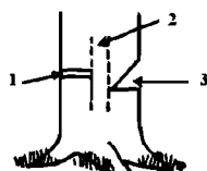
UNDERCUT 3a: 1 back cut 2 holding wood, 3 under cut
